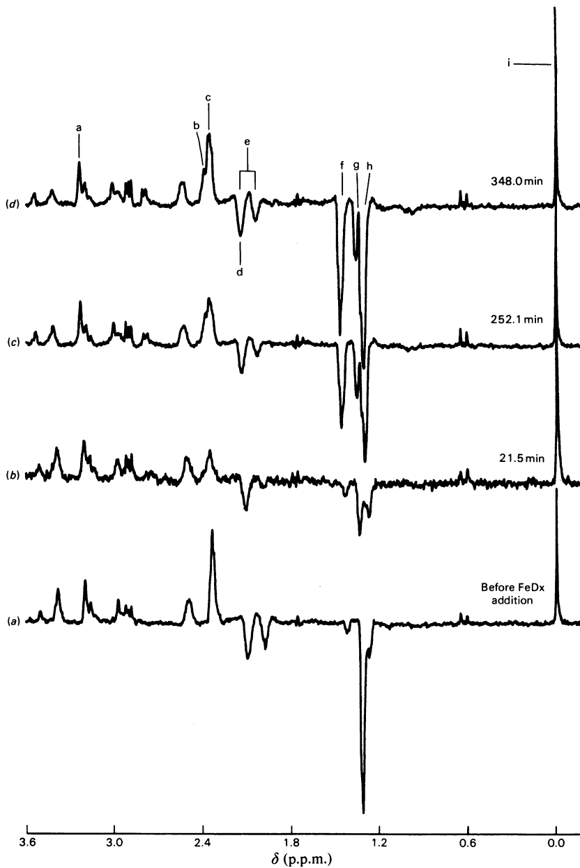
Fig. 6. (a), ^1\text{H-n.m.r. HGSE} spectrum of a suspension of intact erythrocytes (final haematocrit 0.70) to which \alpha\text{-L-glutamyl-L-alanine} was added (final concn. 26.8\text{ mmol/l} of extracellular fluid) at time zero; (b)–(d), time series of ^1\text{H-n.m.r. HGSE} spectra of the same suspension after addition of FeDx ( 1.0\text{ mmol/l} of extracellular fluid) immediately following acquisition of spectrum (a)
