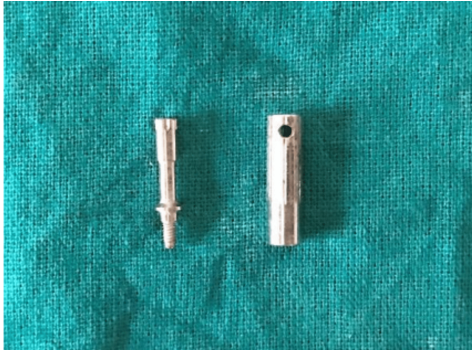
FIGURE 9: Smartpeg of RFA unit
