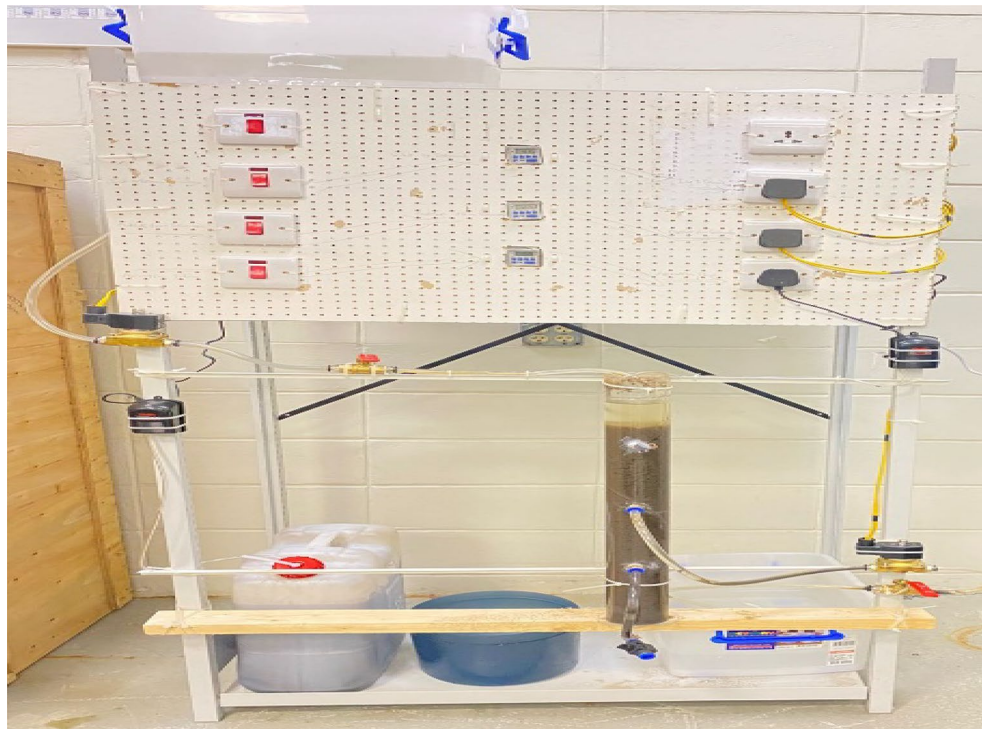
Fig. 1. Lab-scale setup of column-type sequencing batch reactor.
