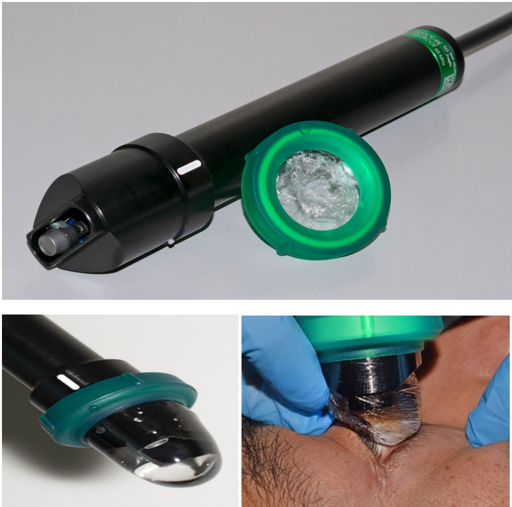
Fig. 1 Image of the 50 MHz Aviso S ultrasound biomicroscopy (UBM) probe with ClearScan cover. Top , Probe with ClearScan cover before assembly. Left , Disposable Clearscan
