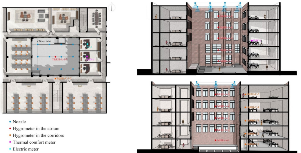
Fig. 2. The schematic diagram of the measurement location in the atrium & the adjust hallway and the monitored offices on the third floor. (Drawn by SketchUp Pro 2021 (21.0.339-64bit) 30 ).
