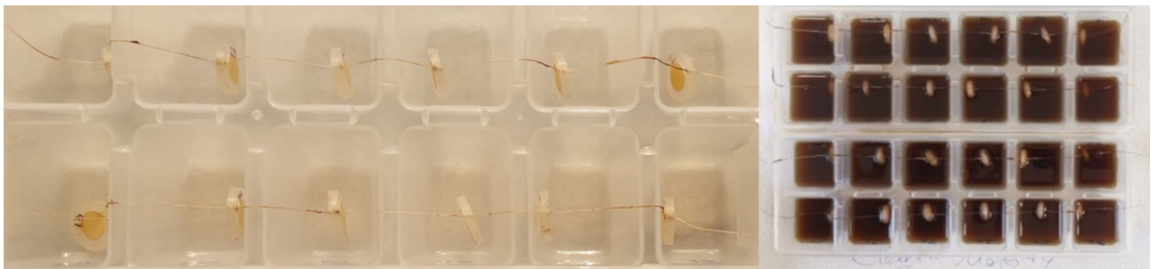
Fig. 3 The specimens were perpendicularly immersed in coffee solution
