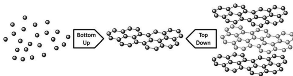
Figure 4. Illustration of top-down and bottom-up synthesis methods of graphene. Reproduced (Adapted) with permission. [22] Copyright 2013, Royal Society of Chemistry.
