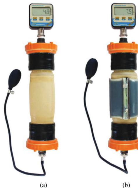
Figure 17. Compression device using electroactive polymer between insulating layers of silicone (dielectric elastomer actuator). Reproduced with permission. [101] Copyright 2018, IEEE.
