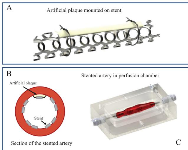
**Figure 4.** A) Ex-vivo study on drug transport from stent to an arterial wall through lipid-free and lipid-rich hydrogels. Artist impression of hydrogel mounted on a stent using sutures. B) Cross-section of a stented artery, showing that part of the stent is in direct contact with the arterial wall and another part through the hydrogel. C) Artist impression of a perfusion chamber mounted with a stented porcine coronary artery.
