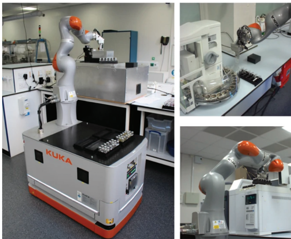
Figure 1. A robotic mobile chemist at work filling vials and loading the gas chromatography equipment. Reproduced with permission. [33] Copyright 2020, Springer Nature.
