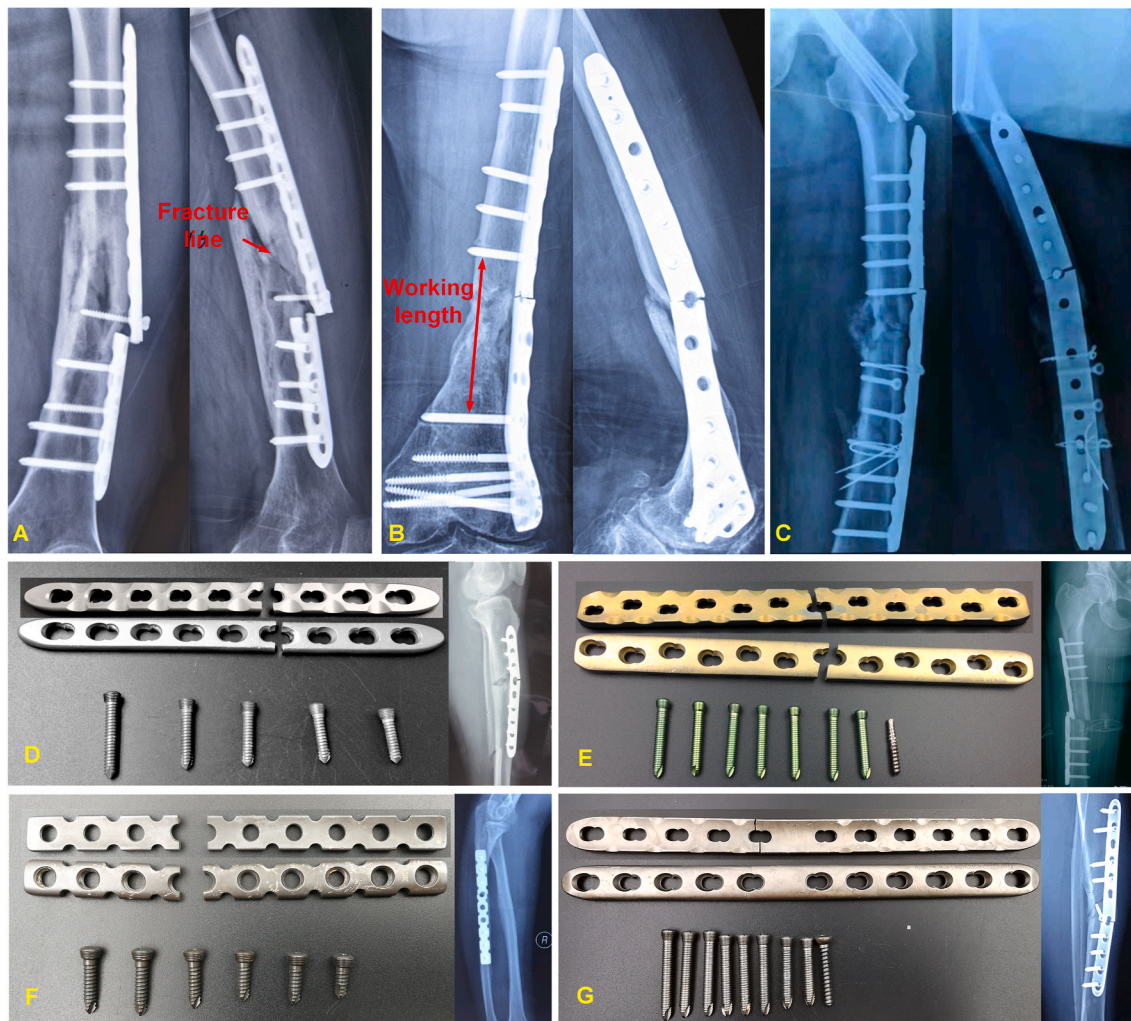
Fig. 1. X-ray of patients and retrieved bone plates. (A) Plate failed at the fracture line (B) Plate failed within the working length (C) Plate failed at the hole posited the screw (D) Traditional plate (E) Asymmetric plate (F) Stress dispersed plate (G) Central enhancement plate.
