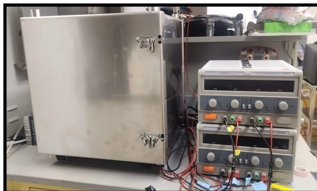
Figure 9. Completed MagShield apparatus. Shown with enclosure safety latches securing the door shut and power supplies positioned next to the mu-metal enclosure so that the leads can reach the coils inside.
