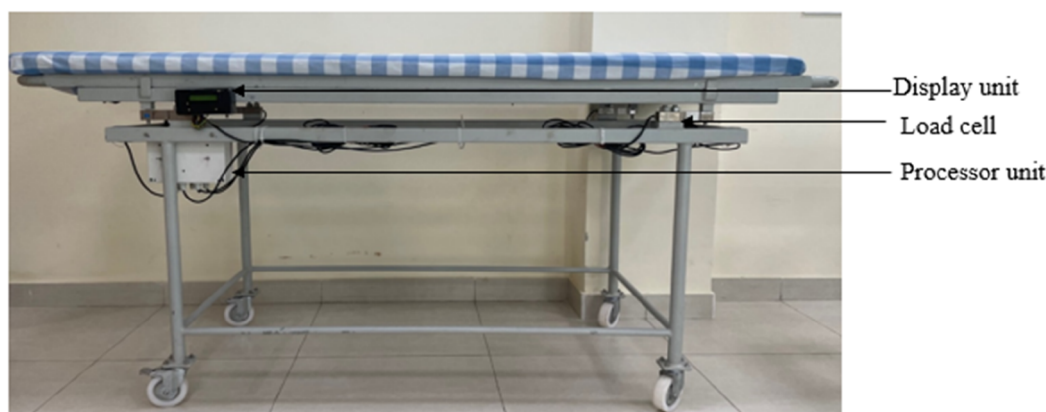
FIGURE 15 Fabricated trolley front view.
