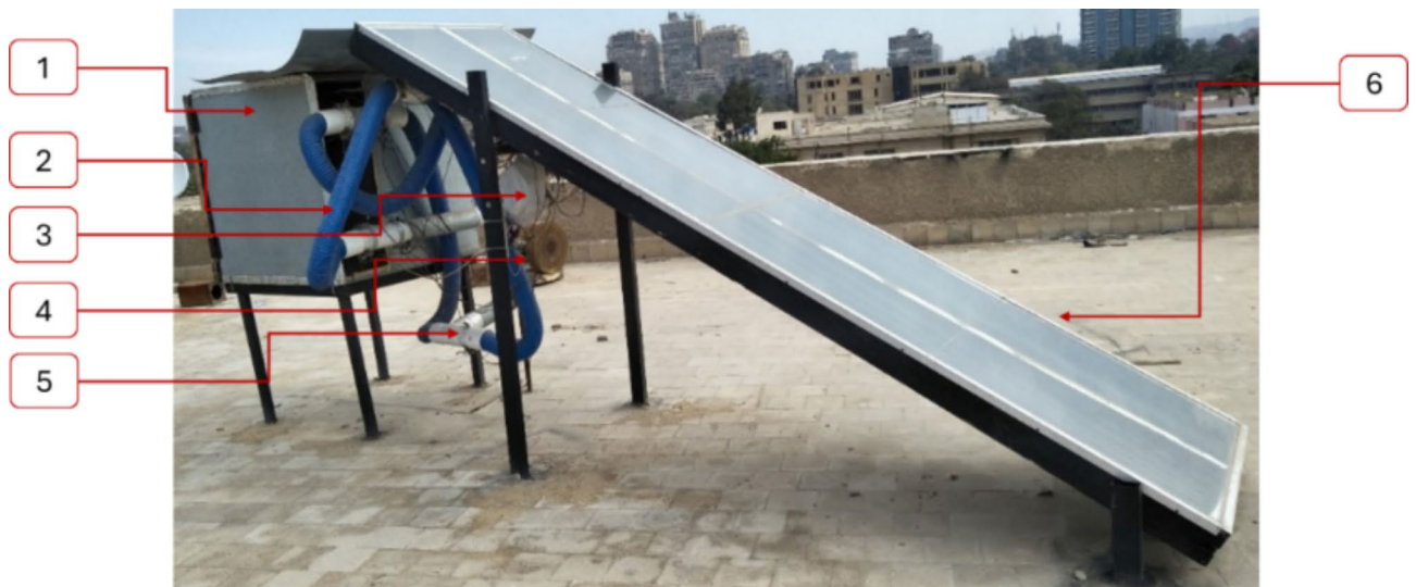
Fig. 1. Main components of the HSD. Whereas (1) Drying room; (2) air pipes; (3) LPG burner; (4) blower; (5) air gates; (6) solar collector 39 .
