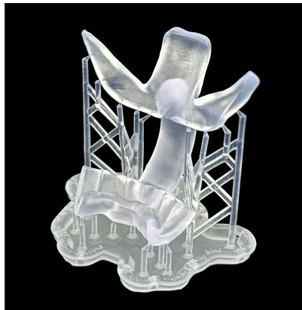
Figure 5. Support structure of a 3D printed cutting guide with SLA technology.
