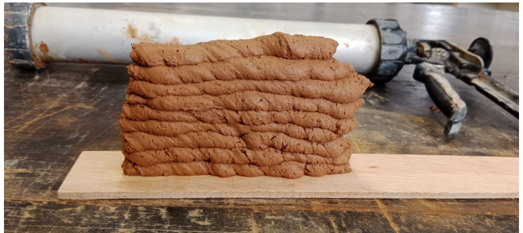
Figure 11. Example of mortar gun extrusion test.
