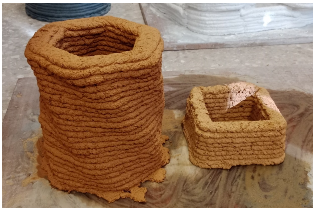
Figure 13. Additive manufacturing pieces printed with the new mortar tailored from clayey sludges.
