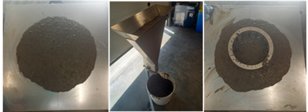
Figure 2. Fresh tests of optimised self-compacting mixes containing sludge-based filler.
