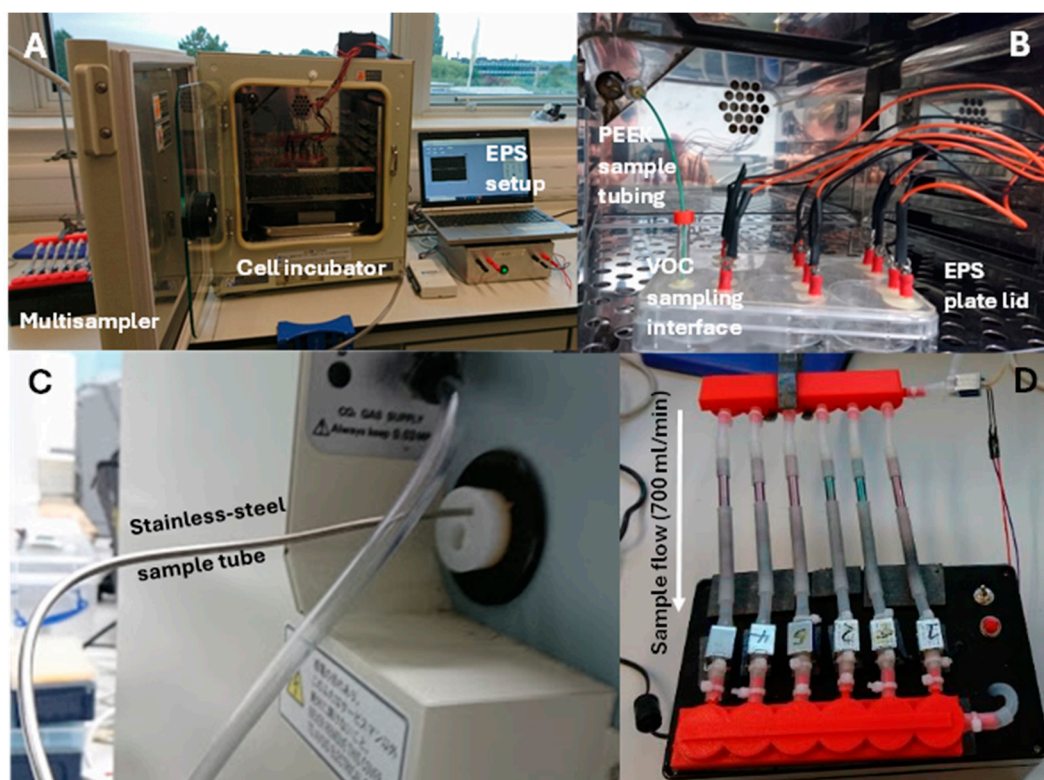
Figure 4. Laboratory set-up for thermal desorption sampling of the headspace of stimulated C2C12 myotubes. (A) Open view of the experimental set up with the multisampler on the left, incubator in the middle and the EPS kit setup to the right. (B) A view inside the incubator of the EPS plate sitting on the top shelf with the PEEK tubing fitted to the VOC sampling interface (clear glass centrifuge vial (12 mm diameter) fitted with a T/S/T septa). (C) Stainless steel sampling tube enters/exits the incubator
