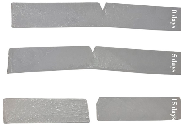
Figure 12. The photography of LDPE samples after impact strength test.
