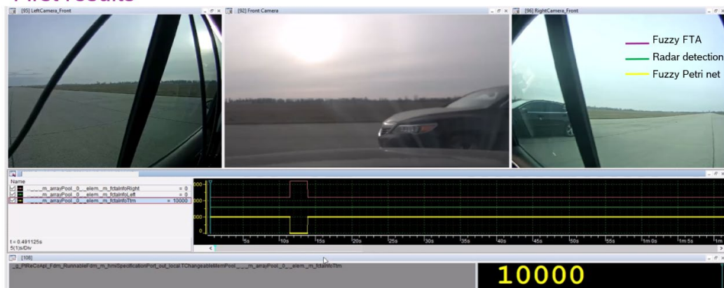
Figure 7. In ID Buzz as an egocar and a car passing through, we look at the reliability of its detection using fuzzy FTA and fuzzy Petri Net.
