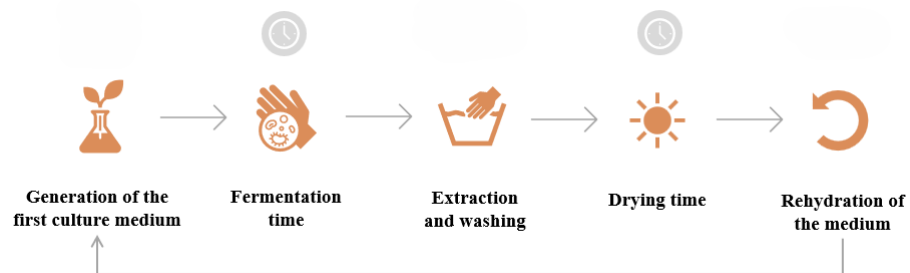
Figure 3. Simplified schematic of bacterial cellulose production with medium reuse. Prepared by the author.
