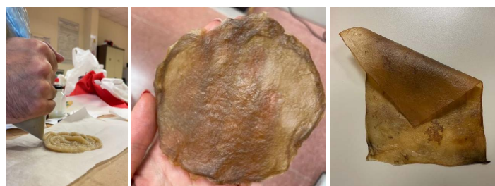
Figure 6. Example of BC extrusion obtained through agitated cultivation for the formation of sheets.
