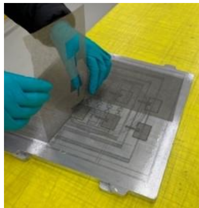
Figure 4. Laser-cut patch antennas prior to electroplating with copper.
