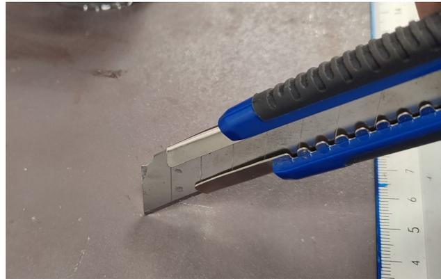
**Figure 3.** Introduction of scoring marks on the steel plate surface.
