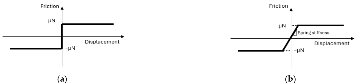
Figure 11. Interfacial contact models that are symmetrical with respect to relative displacement across the interface: (a) Coulomb friction model; (b) linear sliding contact model terminated by frictional sliding, where \mu is the friction coefficient and N is the normal contact force.
