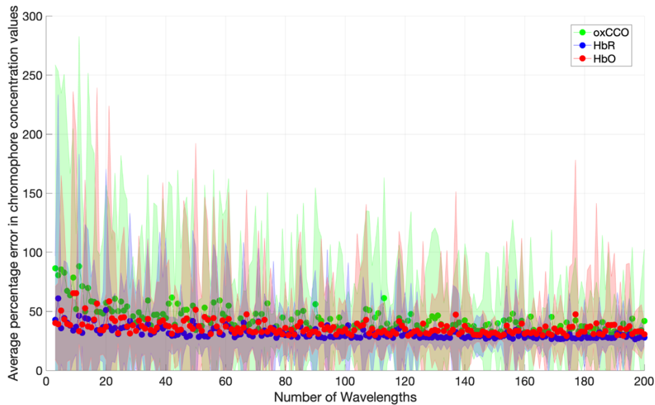
Fig. 6. Graph of chromophore concentration errors against number of wavelengths with a 10% uncertainty in DPF and \square , for Model 2.
