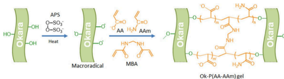
Figure 2. Synthetic route for the preparation of biomass-based Okara-P(AA-AAm) superabsorbent hydrogels. 79
