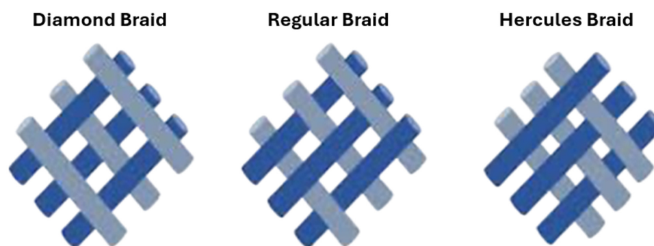
FIG. 11. Three typical tubular 2D braids: Diamond braid features the highest interlacing density with a 1/1 intersection repeat (yarn continuously alternating over and under one yarn). Regular braid follows a 2/2 pattern, and Hercules braid a 3/3 pattern. Reproduced with permission from Doersam et al. , Adv. Mater. Technol. 7, 2101720 (2022). Copyright 2022 Authors, licensed under a Creative Commons Attribution (CC BY) License.
