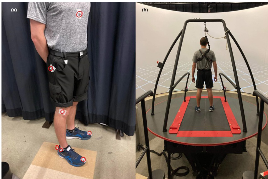
FIGURE 3 Subject (a) with eleven infrared reflective markers circled in red and (b) on the CAREN (Computer-Assisted Rehabilitation Environment) platform at the beginning of an experiment.
