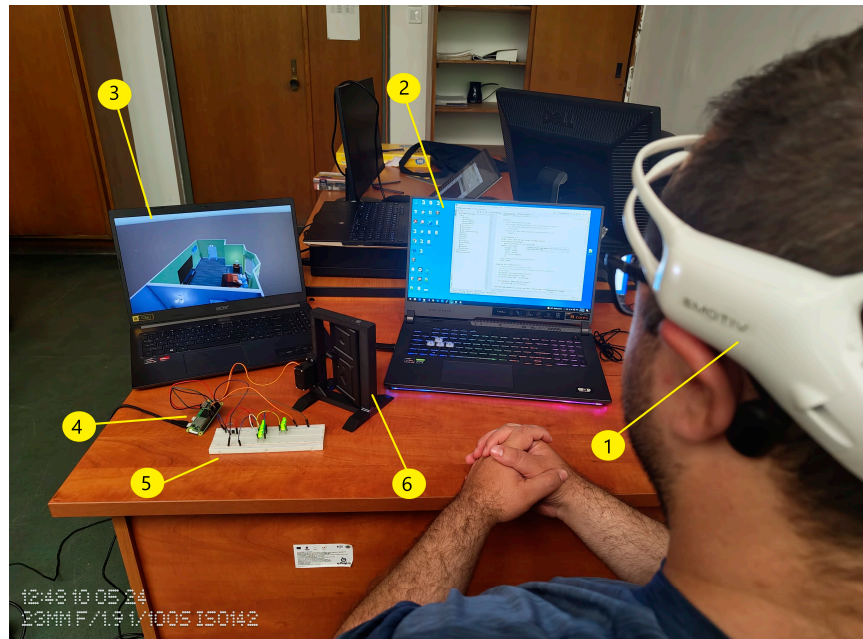
Figure 1. Real-time home automation system and video simulation: 1. EMOTIV Insight neural headset. 2. Cortex API and FastAPI server are running. 3. The simulated system (Unity Engine). 4. Raspberry Pi Zero 2 W. 5. BreadBoard with 5V LEDs. 6. PLA Door and frame, equipped with Digital MG996 servo motor.
