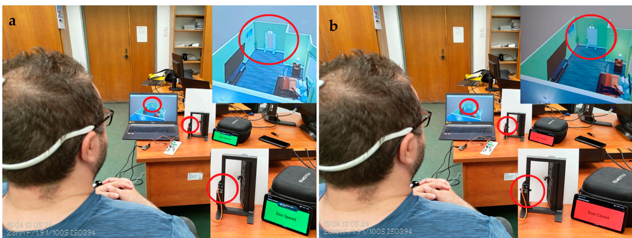
Figure 19. Lock and unlock the door using brain signals, with real-time notifications on video simulation and phone: (a). Door unlocked; (b). door locked.
