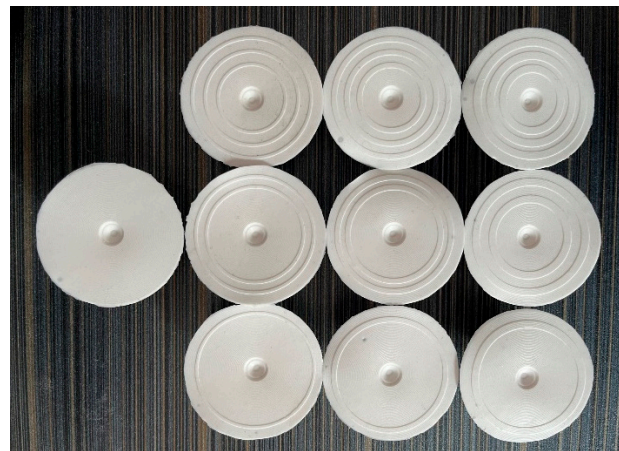
Figure 6. The standard and bionic suckers.
