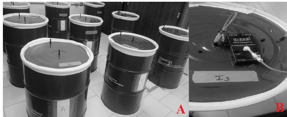
Figure 1. Metallic drums used for fumigation (A) and Silo-Chek—Canary Co device (B).
