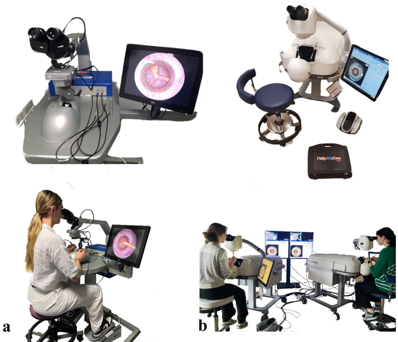
Fig. 1. Virtual reality simulators. (A) EyeSi© (EYS) is a computer system with a microscope-like display for 3D visuals. It features a table setup with a mannequin head, a simulated eye, two control pedals for microscope and phacoemulsification operations, and a tactile interface with three ophthalmic probes. (B) HelpMeSee© (HMS) is a virtual reality simulator with tactile feedback, resembling a reclining patient connected to a microscope-shaped screen for 3D visuals. The setup includes a table, a mannequin head with tactile feedback, a single pedal for phacoemulsification control, and a tactile interface with two ophthalmic probes that mimic the surgical instruments.
