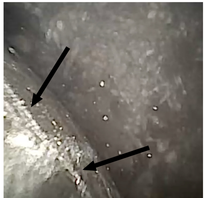
Figure 5 Humeral component grinding traces.
