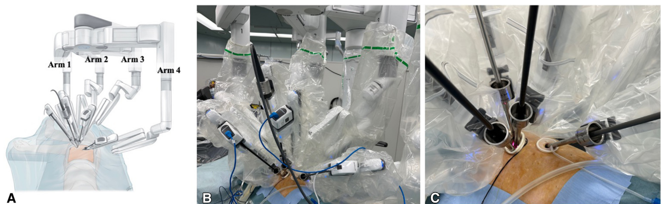
FIGURE 2. Left-side configuration. A, Illustration showing the port placement and setup of robotic arms on the left side. Arm 1 is used for the left hand, arm 2 is used for the camera, arm 3 is for the retraction, and arm 4 is for the right hand. B, The camera is normally placed in the posterior part of the incision to allow the other robotic instruments working below the camera in the same incision to be parallel along the sagittal plane. C, Enlarged view of the port placement. Arm 3 is used for the retraction as is the role of the assistant in original dual-portal RATS. This retraction arm is very helpful in obtaining better exposure. Arm 1 and arm 4 robotic instruments are used through another incision that opens wide toward the ventral side to prevent interference.
