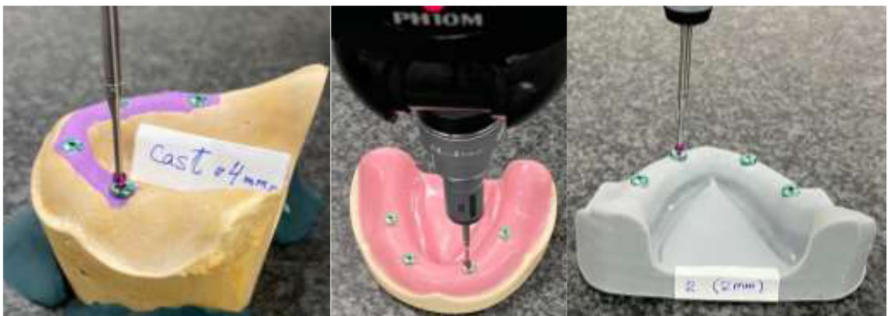
Fig. 5 Reference models, stone cast and printed cast measurement on CMM
