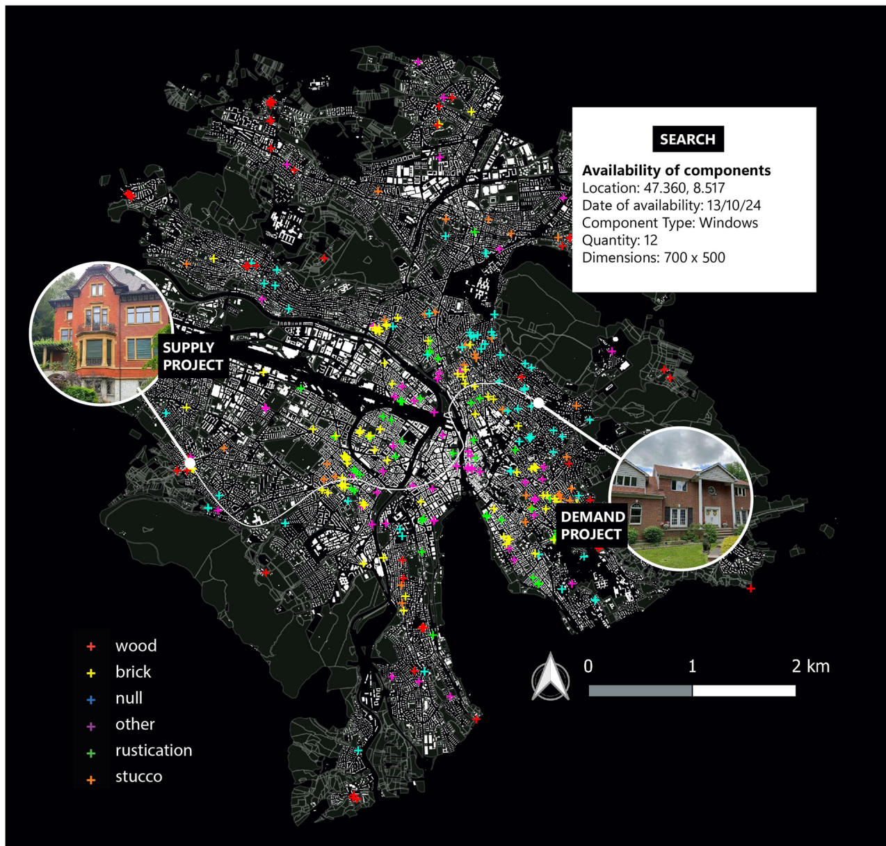
Fig. 2 | Spatial distribution of building materials for a subset of buildings in Zurich, Switzerland, adapted from ref. 88.
