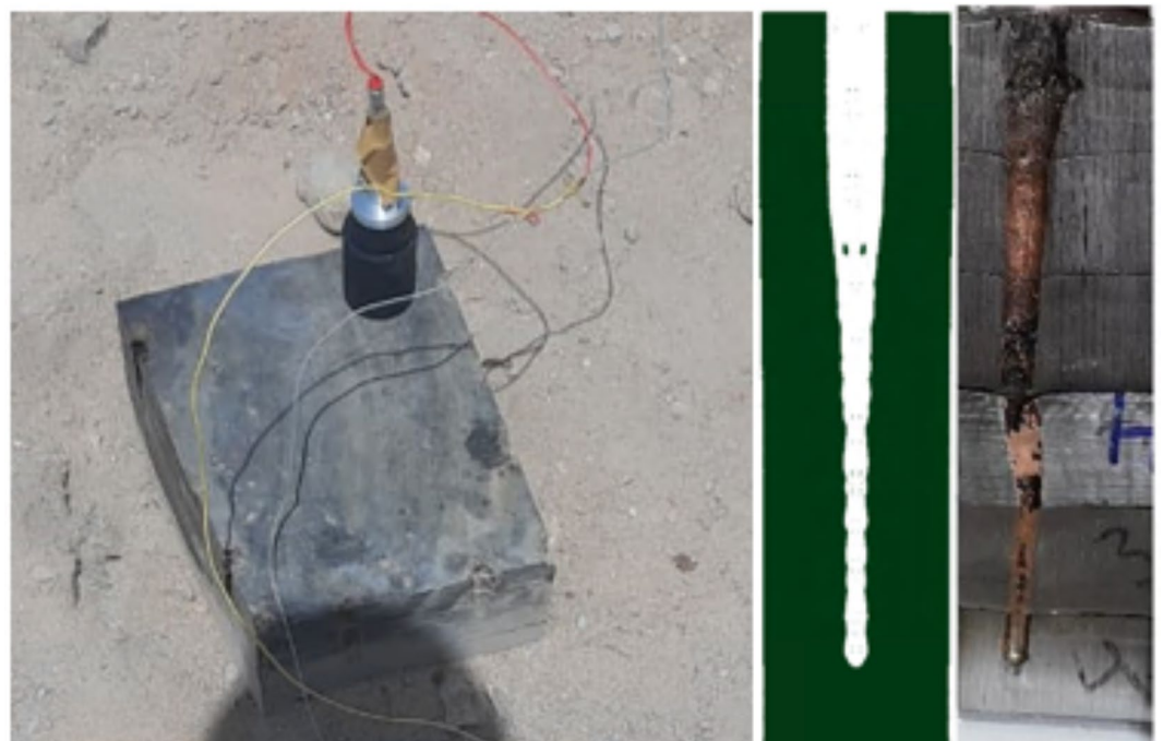
Fig. 18. The penetration test setup (left), the real HMX-V5 shaped charge jet penetration crater profile (right) and numerical one (middle).
