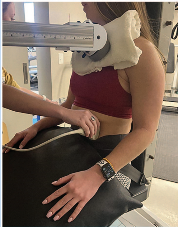
Figure 2. Subject testing position with the use of the static dynamometer.
