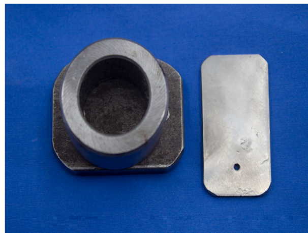
Fig. 2. Stainless split mold for sample preparation.
