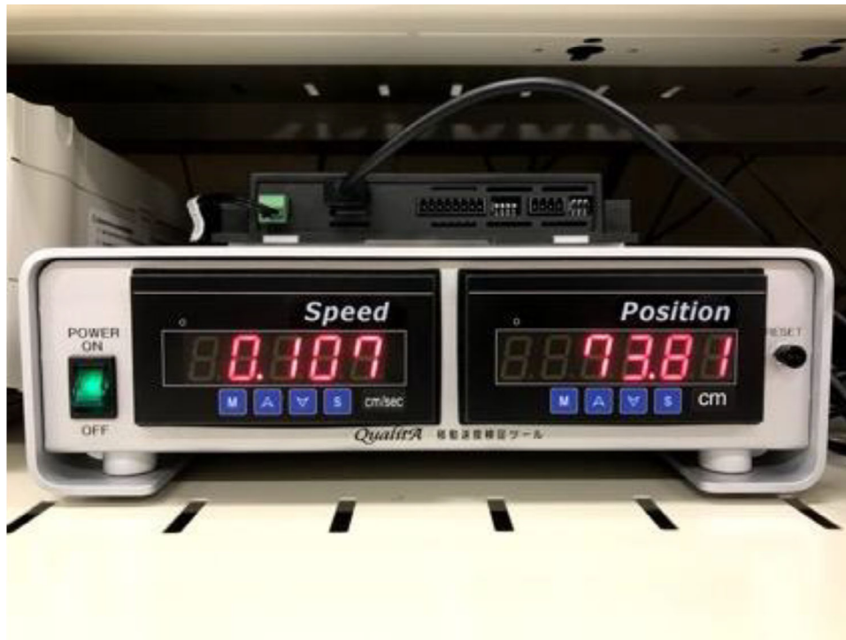
FIGURE 4 Monitor display when a plan with a couch speed of 1 mm/s is executed.
