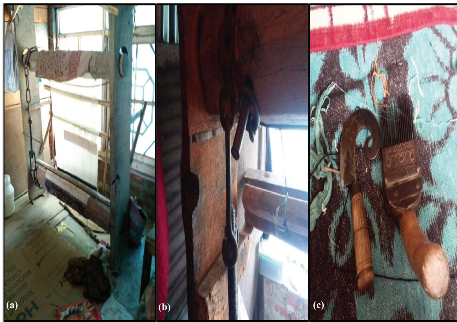
Figure 2. Figure 2 (a) depicts a wooden loom; Figure (b) displays the chain of the loom; Figure (c) shows khor and panje. Source: fieldwork
