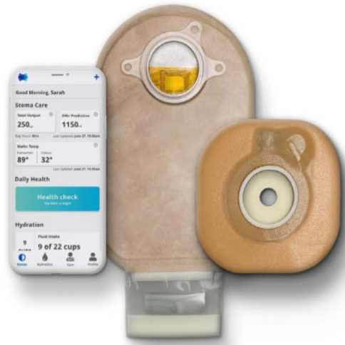
Figure 20. Alfred Smart Bag device, where the mobile application and the two-piece bag are visible, with the implementation of resistive/capacitive sensor arrays, calculating the amount of waste in the bag. Figure authorized by the editor [55].
