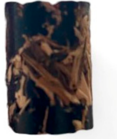
Figure 13. The product of the hemp compaction process with 50% ABS regranulate share and 0–4 mm of shives fraction.
