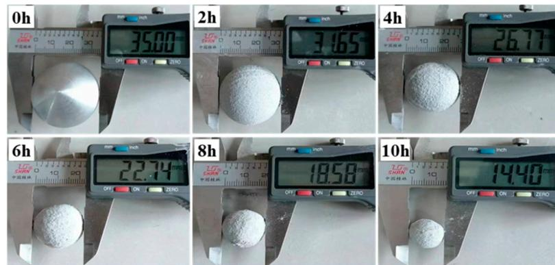
**Figure 13.** Dissolution diagram of as-cast Al-Mg-Ga-Sn-In soluble aluminum alloy spheres with an elemental Mg content of 3.0 wt.% in water at  $90\text{ }^{\circ}\text{C}$ .
