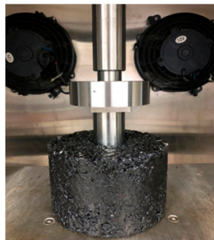
Figure 5. Loading diagram of uniaxial penetration test.
