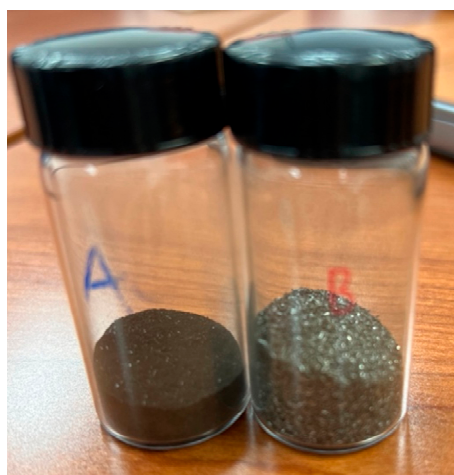
Figure 5. Samples from the (A) innermost and (B) outermost layers from the Inconel reactor used in the reactions.
