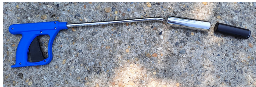
Figure 2. The applicator with the waterproof enclosure of the bolus.
