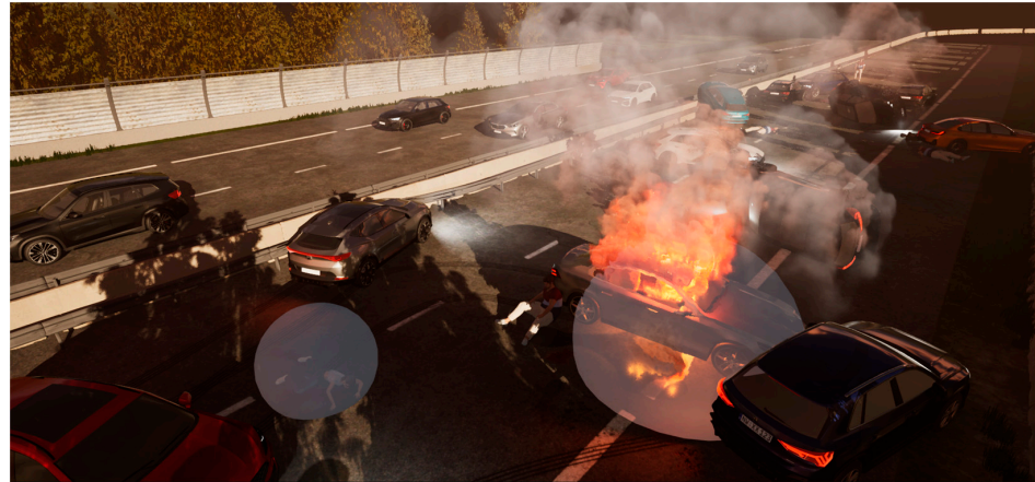
Figure 10. VR scenario implemented in Unreal Engine (© Thera Bytes). Circular gray areas (bubbles) automatically control the fragrance pumps via the communication interface, as presented in Figure 9.
