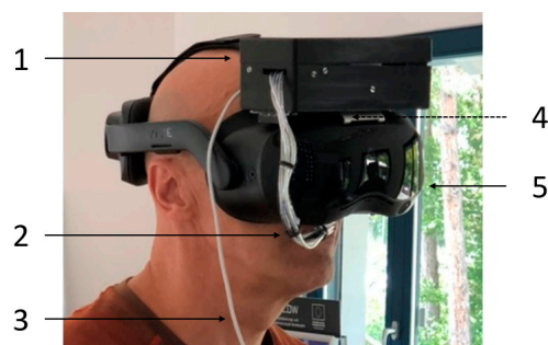
Figure 8. Head-mounted device including the developed prototype (1) of the odor delivery system with micropumps and the VR headset (5), which is attached to an aluminum plate (4). Odor/air mixtures are transported close to the human nose via PTFE tubes (2). The prototype version shown in this figure uses a cable connection (3) for power supply and communication.
