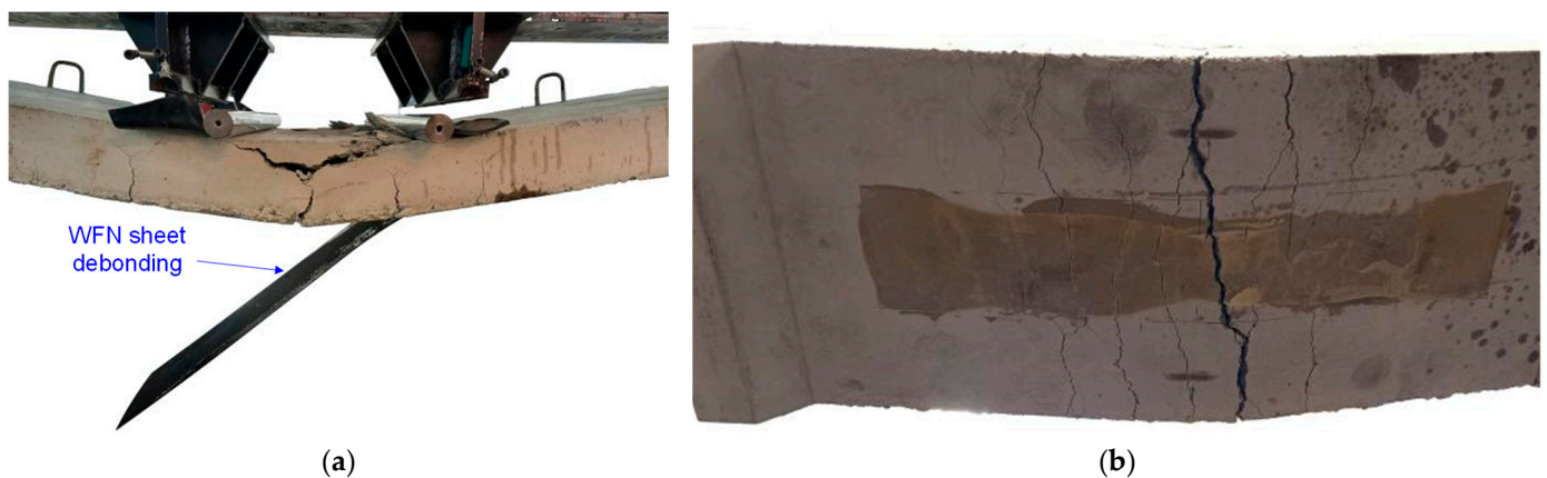
Figure 13. Cracks and the failure mode of slab strengthened by recycled WS. (a) Front view and (b) bottom view.
