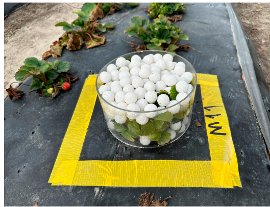
Figure 5. An acrylic cylindrical case with a strawberry plant filled with EPS balls to calculate the volume difference between the number of balls with and without plants.
