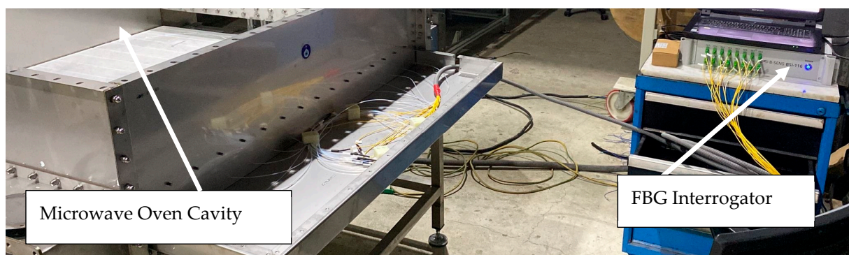
Figure 8. Measurement setup with the instrumented microwave oven on the left and the BSI-116 data acquisition system on the right.
